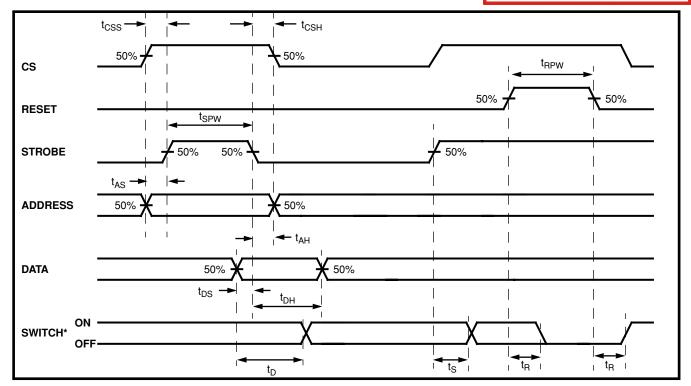
Figure 3 - Control Memory Timing Diagram
