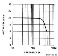
$V_{O(DC)} = 5.4V$ Differential phase error <  $0.5^{\circ}$ Differential gain error < 2% $f_{-3~dB}$  low = 2.5~Hz
