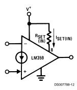
$$I_{SET(IN)} = \frac{V^+ - V_{BE}}{R_{SET(IN)} + 500\Omega}$$
