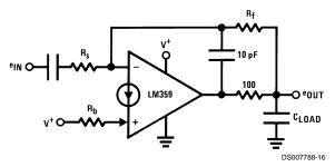
FIGURE 11. Isolating Large Capacitive Loads
