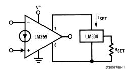
$$I_{SET} = \frac{67.7 \text{ mV}}{R_{SET}} @25^{\circ}\text{C}$$
