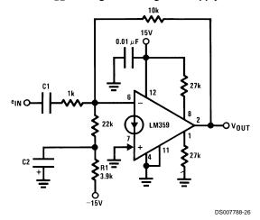
R1 and C2 provide additional filtering of the negative biasing supply
