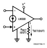
$$I_{SET(OUT)} = \frac{V^+ - V_{BE}}{R_{SET(OUT)} + 5000}$$
