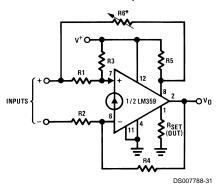
$$V_{\text{O(DC)}} = \frac{\text{R4}}{\text{R3}} \left( V^+ \, - \, \varphi \right) \text{ where } \varphi = 0.6 V$$
