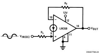
$$\begin{split} V_{O(DC)} &= V_{BE}(-) + \frac{(V_{IN(DC)} - V_{BE}(+)) R_f}{R_s} \\ A_{V(AC)} &= + \frac{R_f}{R_s + r_o(+)} \end{split}$$
