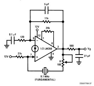
$V_0 = 500 \text{ mVp-p}$  f = 9.1 MHzTHD < 2.5%
