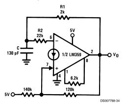
$$\label{eq:f_total_fit} \begin{split} f &= 1 \text{ MHz} \\ \text{Output is TTL compatible} \\ \text{Frequency is adjusted by R1 \& C (R1 } \leqslant \text{R2}) \end{split}$$
