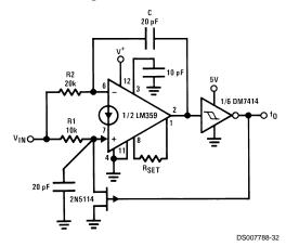
$$\begin{split} f_0 &= \frac{\sqrt{IN - \phi}}{4 \, \text{C} \Delta \text{V} \, \text{R1}} \\ \text{where: } R2 &= 2 \text{R1} \\ \phi &= \text{amplifier input voltage} = 0.6 \text{V} \\ \Delta \text{V} &= \text{DM7414 hysteresis, typ 1V} \end{split}$$
