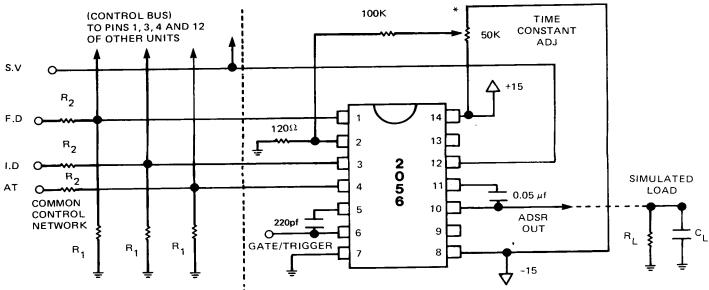
\*Optional: Adjusts for capacitor value and slight unit to unit variation. Ground Pin 2 if not required.
