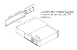
③ Set the Protect Switch on the Memory Cartridge to the OFF position.
