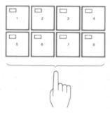
To select other variation of that voice, hold the Bank Button down and push the corresponding Voice Selector Button. Here, the Voice Selector Buttons 1 to 8 correspond to the bank numbers.
