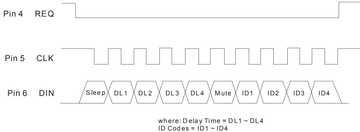
The DIN Signal is shifted in the falling edge of the CLK Signal when the ID Code Bits values are verified as follows:
