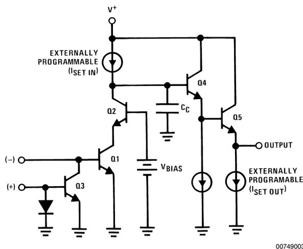
FIGURE 3. A Simplified Schematic of the LM359, a High Speed, Current Differencing Amplifier. The Input, Output and Speed Characteristics are Externally Programmable.
