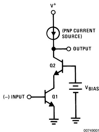
FIGURE 1. Basic Cascode Circuit
